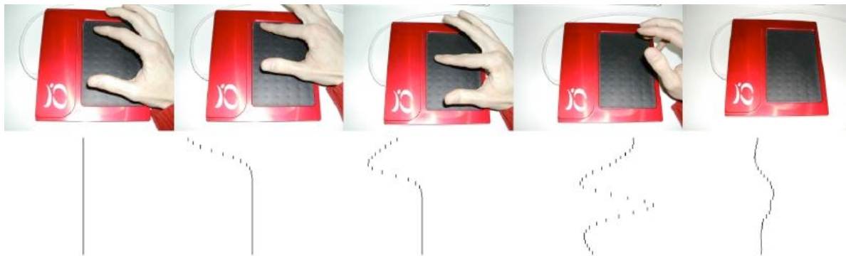
Fig. 9. When the user presses the surface, the forces applied cause the string to leave the equilibrium state; after being stimulated and driven by the graphical tablet, the string will evolve according to its own dynamics, before returning to its initial position.
